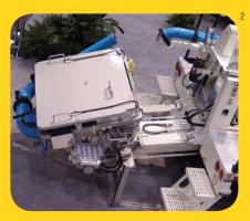
Fully removable, Putzmeister's modular bolt-on flatpack and hydraulic system combine versatility and servicing convenience. Pump cells can be switched out as jobs require or when maintenance is necessary. This feature also provides easier access to the S-Valve and shift cylinders.
